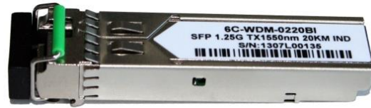
1000Base-BX WDM Singlemode (TX 1550 nm – RX 1310 nm)
