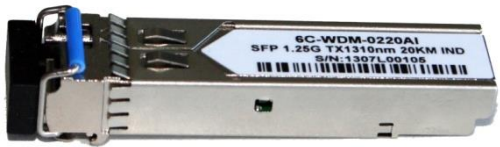
1000Base-BX WDM Singlemode (TX 1310 nm – RX 1550 nm)
